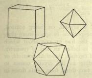
FIG. 5.—SIMPLE CUBE AND SIMPLE OCTAHEDRON. A COMBINATION OF THE CUBE AND OCTAHEDRON AS FOUND IN CRYSTALS OF GALENA.
